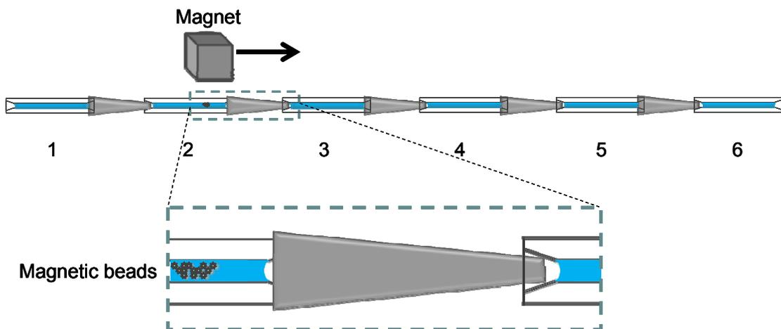
**Figure 3.** Capillary chambers were arranged sequentially on a horizontal stage. Sample lysate with lysis buffer and magnetic beads are added to the first chamber. As a magnet is moved over the exterior of the capillaries the magnetic beads are pulled through the chambers and transfers the beads to chamber 6. This process washes, rinses and elutes RNA from the sample lysate.
