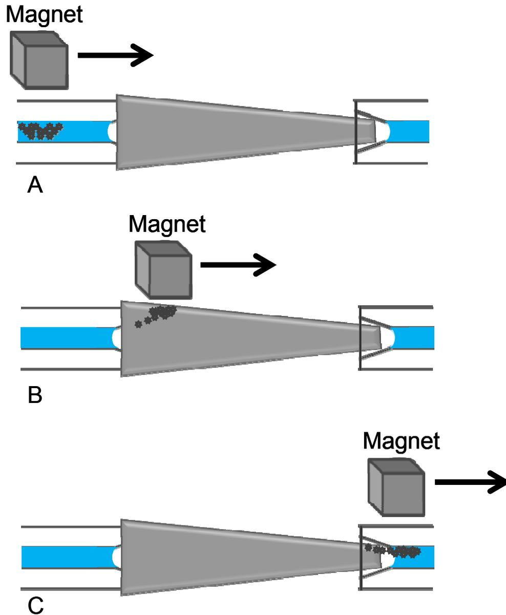
**Figure 4.** The beads follow the magnet as the magnet is moved from left to right. The small capillary diameter which creates high surface tension and the air spacers allow for movement of the beads from one capillary to the next without transferring buffer from one capillary chamber to the next.
