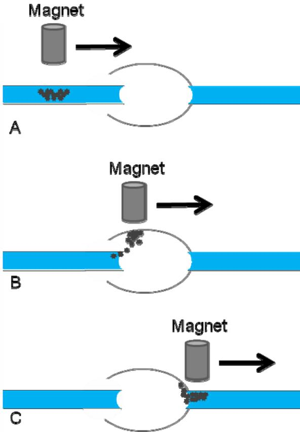
**Figure 2.** The beads follow the magnet as the magnet is moved from left to right. Blue represents the processing solutions and the air spacers between them allow for movement of the beads from one capillary to the next without transferring solutions. The retention of the solution is due to surface tension holding the solution within the capillary chamber.
