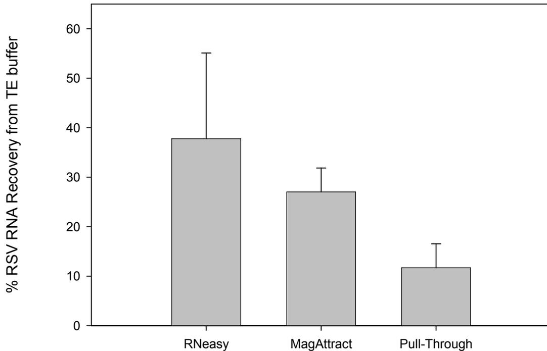
**Figure 5.** Comparisons were made of the number of copies of RNA per  $\mu\text{L}$  before and after extraction from TE buffer. The percent recovery was calculated by dividing the copy number values for each extraction method by the copy number obtained before extraction. Tests were run in triplicate and shown as means  $\pm$  standard deviation (N=3).
