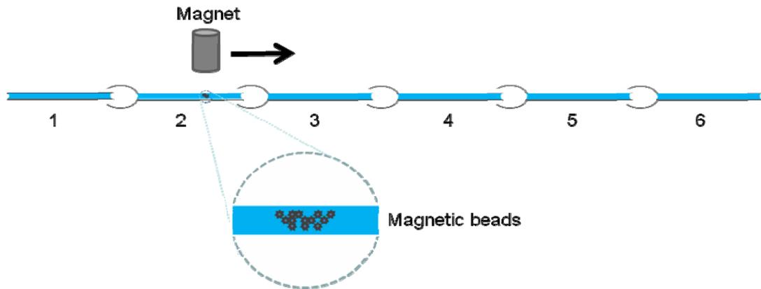
**Figure 1.** Capillary chambers were arranged sequentially on a horizontal stage. Sample lysate with lysis buffer and magnetic beads are added to the first chamber. As a magnet is moved over the exterior of the capillaries the magnetic beads are pulled through the chambers and transferred to chamber 6. This process washes, rinses and elutes RNA from the sample lysate.
